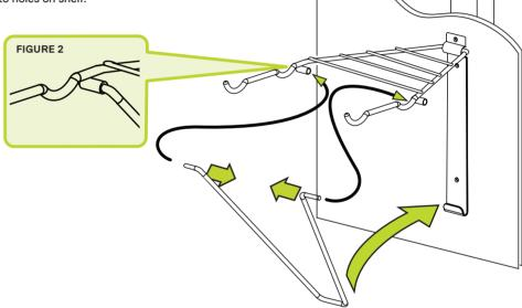
Make sure that shelf support is securely placed in bottom of wall bracket. (Figure 3)
